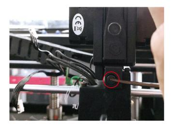
Install the 2 original rear screws with the 2.5mm hex wrench. Do not tighten the screws fully.
