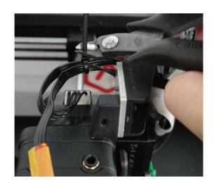
Secure the wires underneath the motors with another cable tie.
