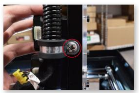
Lastly, remove the two fixing screws and cover from the extruder board.
