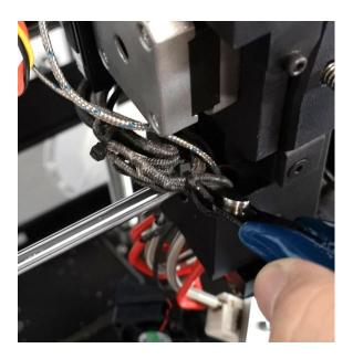
Loosen the screws marked in following image. And remove the Heating Rod cables from extruder board.
