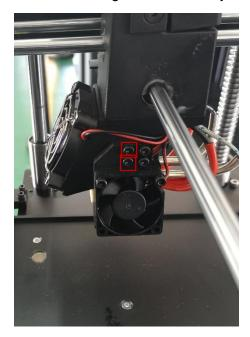
• Loosen the fixing screw marked in red with 2.5mm hex wrench.
